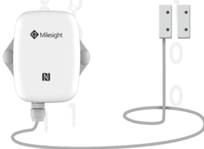
EM300-MCS As EM300-TH plus magnetic contact switch
